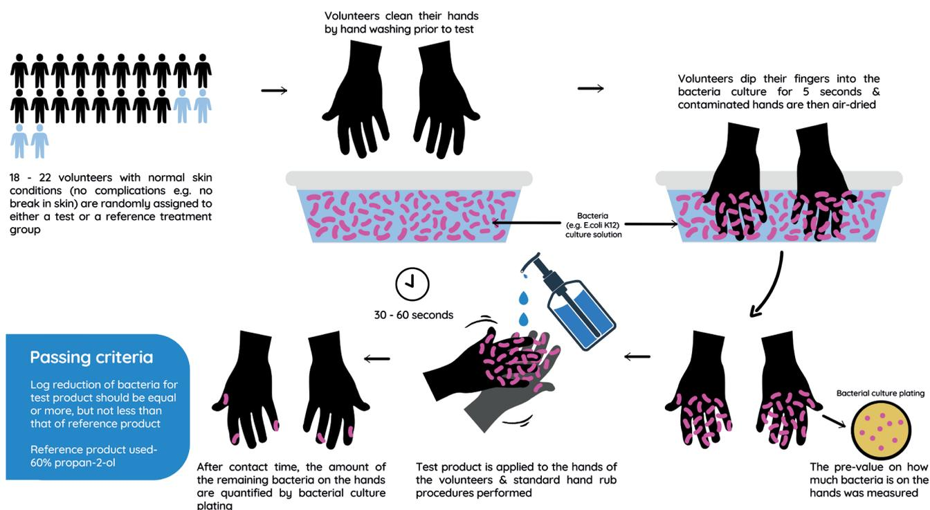
Figure 1. How is EN1500 being carried out?
